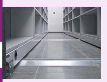
The trackage is galvanized. The total height of the track is 12 mm. Trackage is anchored to the floor with expansion bolts. The outermost tracks have an anti-tilt system, protecting against overturning. Optimally selected number of rails ensures smooth and easy movement of units. There is also a possibility of installing a chain in the trackway.
