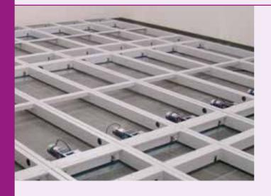
The frame is made of steel profiles powder coated in RAL 7035 colour. The frame is equipped with shafts and cast iron wheels. The wheels have ball bearing to improve the quality of use. The frames are equipped with rubber distance buffers in order to prevent units from sliding off. Movable shelving provide the possibility of transmission by means of following elements: electric motor, cogwheels coupled with transmission shaft.
