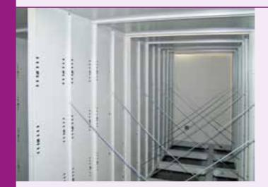
Load-bearing wall is made of powder coated steel, perforated every 25 mm (either in intervals or continuously). Thus shelves can be adjusted at any desired height. For additional rigidity of units, a cross-wise strengthening is applied.
