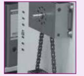
Solid crank mechanism - big transmission, easy to move.
